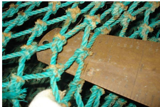
Figure 6-6 Measure stretched mesh opening from the inner edge of knots (upper left; modified from Ferro and Xu 1996) using a wedge gauge (upper right; Fonteyne et al. 2007). Bottom image supplied by S. Sei (Sierra Leone).
