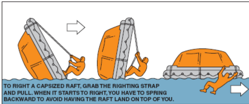
Figure 15-11 Righting the life raft. Wind direction represented by the arrows. Image from (Transport Canada 2003).
